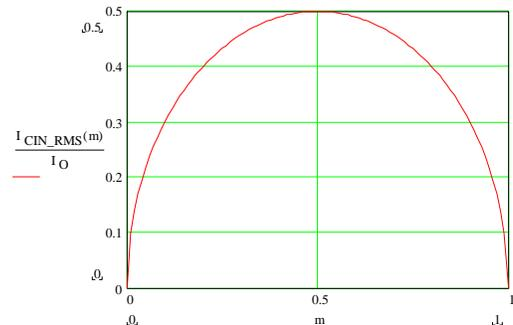
Figure 2. I<sub>CIN</sub> vs. voltage conversion ratio
