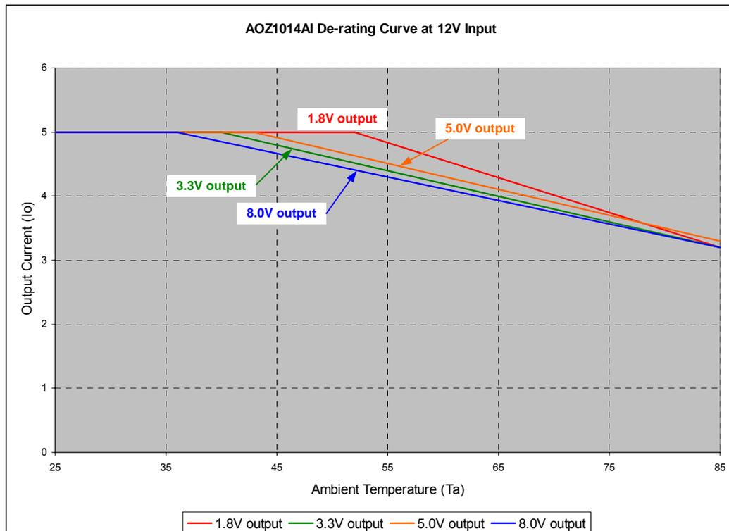
**Thermal de-rating curves for DFN-8 package part under typical input and output condition**
